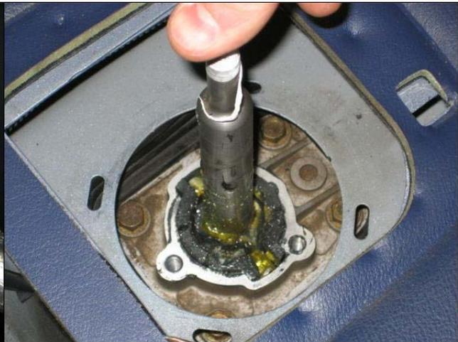
10. Place the retaining collar over the shifter and line up the bolt holes. Notice the orientation of the indentation on the inner surface of the collar points toward 6<sup>th</sup> gear.
