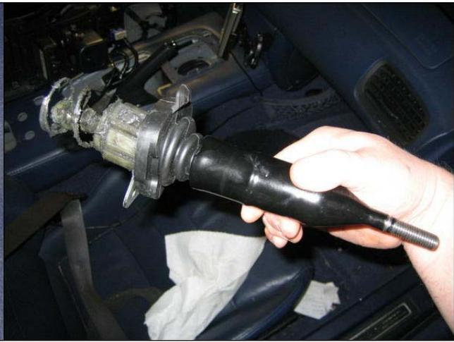
8. Pull the spring off the end of the stock shifter and install it onto the short shifter.
