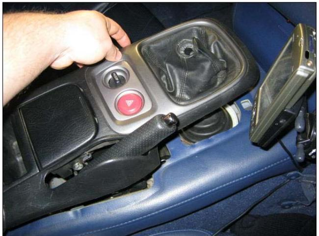
4. Remove the grey foam from the transmission tunnel, and remove the rubber shifter boot. Use a screwdriver at the corners of the tunnel opening to release the 4 clips on the underside of the white plastic ring.
