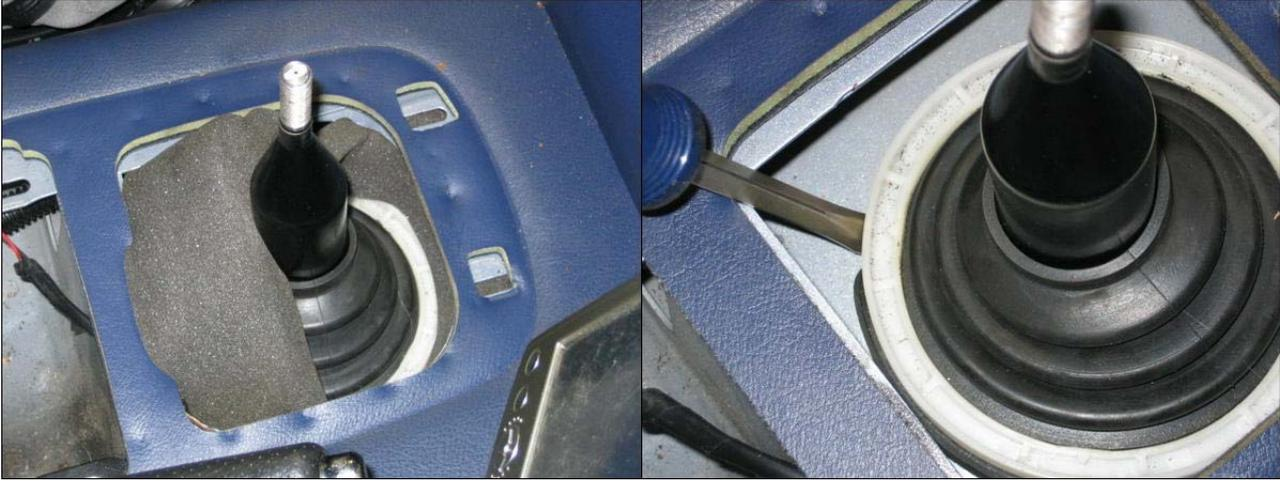
5. Pull the rubber cover up and twist it around to expose the (3) 10mm bolts
