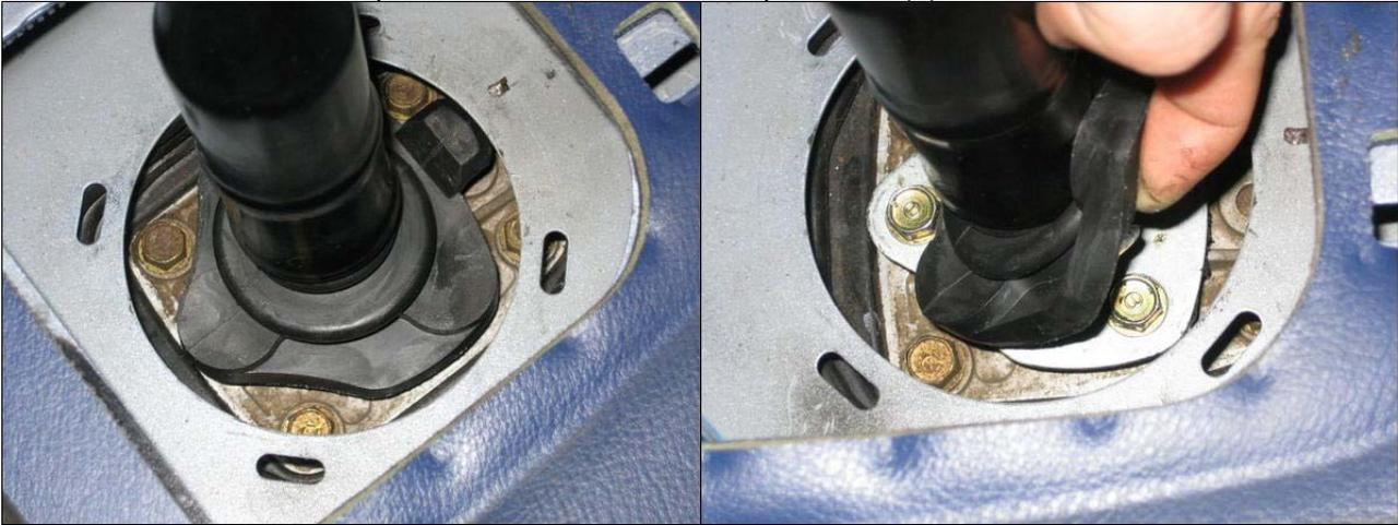
6. Remove the 10mm bolts on the retaining collar
