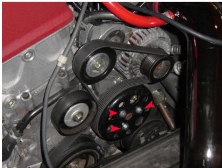
**Figure 9 Water Pump Pulley**
