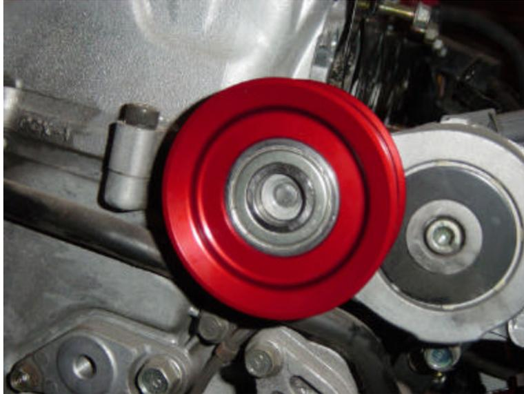
**Figure 4 Auto-Tension Pulley Replaced**
