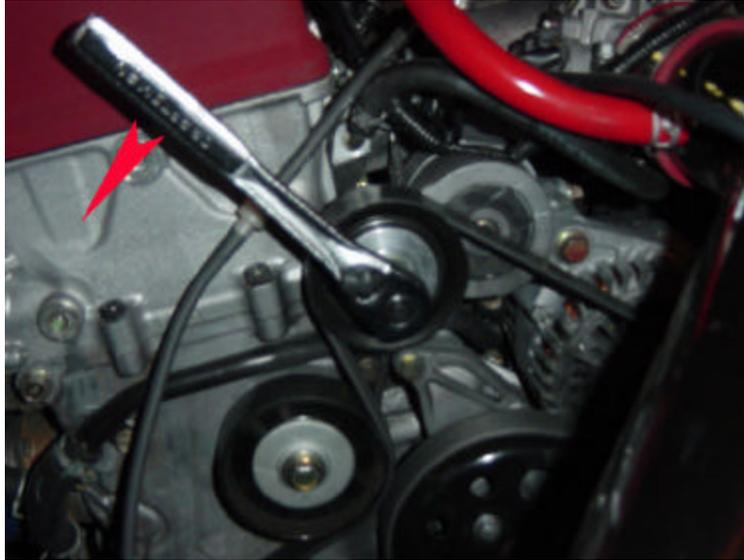
Figure 2 Auto-Tension Pulley
