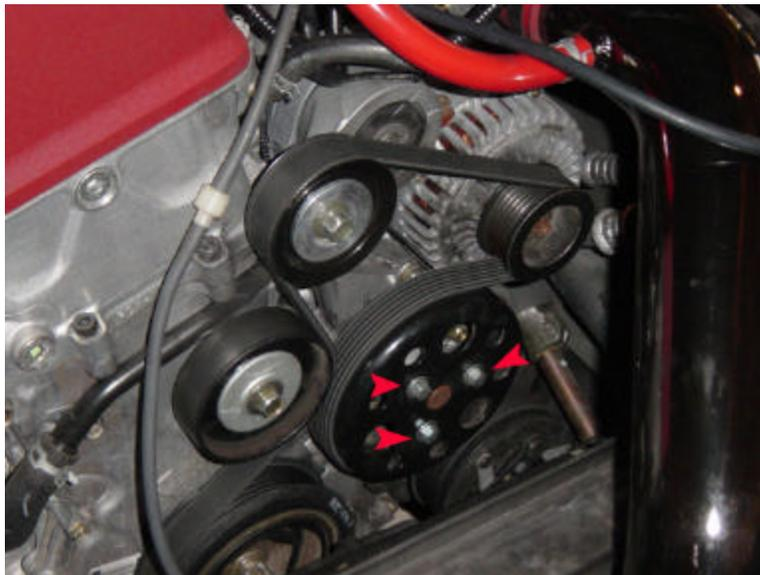
**Figure 1 Water Pump Pulley Bolts**
