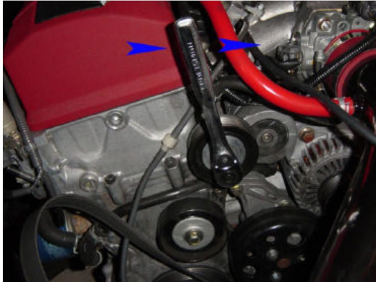
Figure 3 Auto-Tension Pulley Removal
