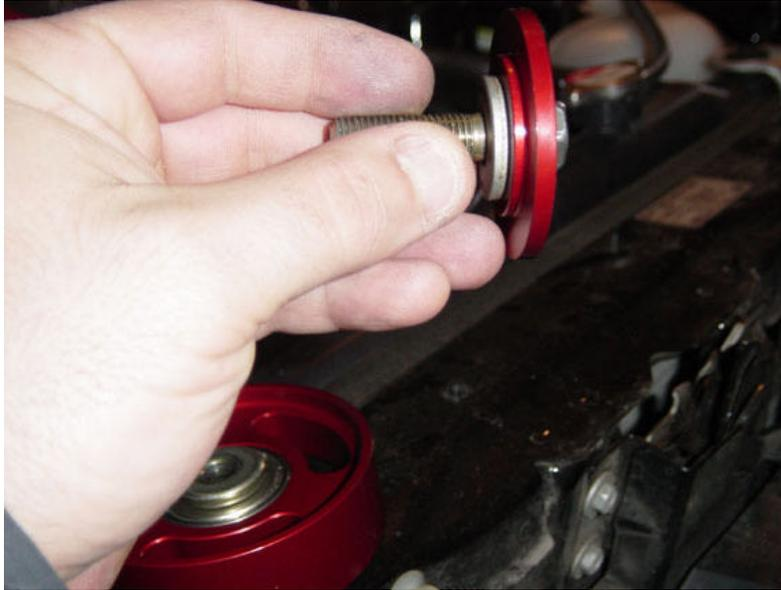
**Figure 8 Idler Pulley Bolt**
