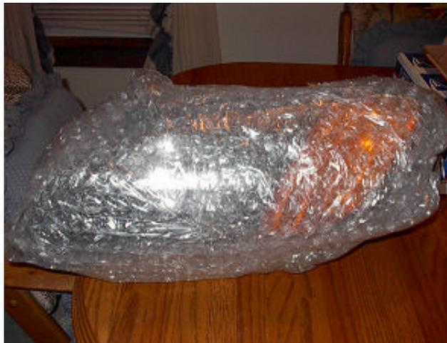
**Figure 13 Bubble Wrap each assembly**
