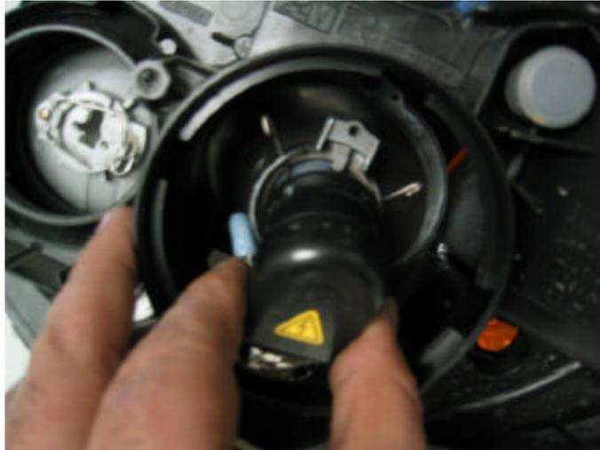
**Figure 7 Pull to Remove**
