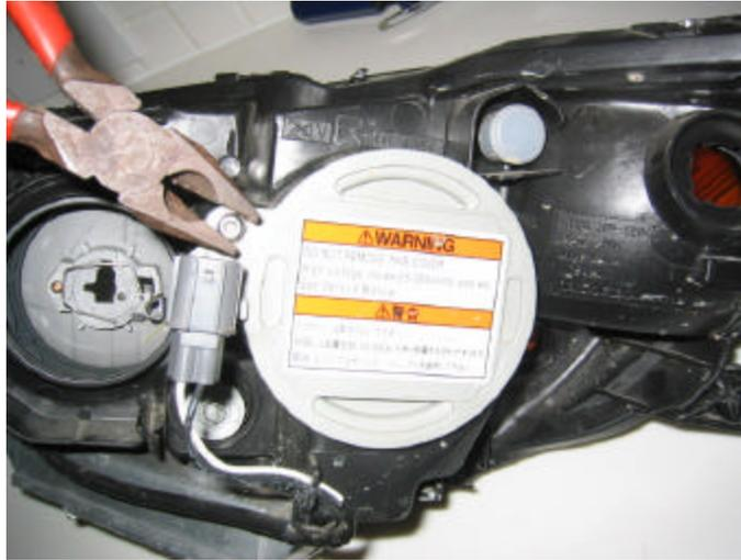
**Figure 4 Security Screw Removal T25**
