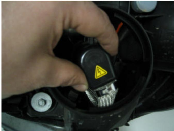
**Figure 6b HID Socket (Unlocked)**
