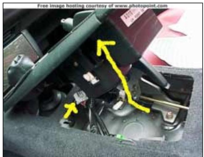
4. Being careful not to scratch the brake handle, remove the plastic assembly from the center console and set aside in a safe place. At this time, check to see that all six metal spring clips are still attached firmly to this part.
