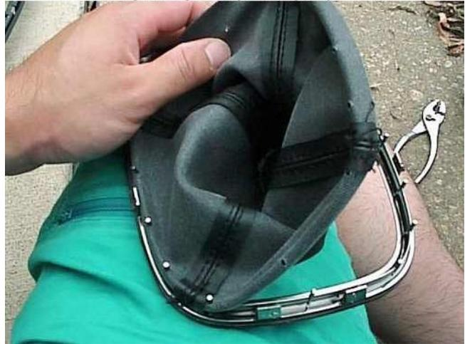
9. Mount the new leather boot, fitting the holes in the boot over the plastic posts on the mount. **Again, take care not to break the posts.**
