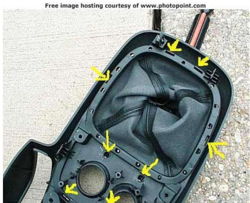
Start with the anchors shown near the bottom of the picture and loosen that part of the assembly first. To loosen these tabs, squeeze them with a pair of needle nose pliers and push them out.
