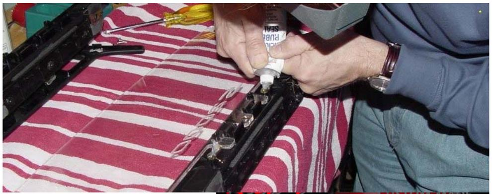
get any of these glues on the screen. Wipe them off immediately if you do. This gluing is critical to the integrity and durability of the of the mechanism and screen, so be sure to do the job right to ensure that the mechanism is solidly glued together.
