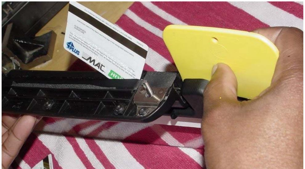
8. With the pieces apart, remove the three screws that hold the windscreen to the mechanism. Place the screws in a safe place for use in reassembling the mechanism. Then clean all of the old glue out of the four slots and matching tabs. Use a watchmakers screwdriver and needle nose pliers to do this
