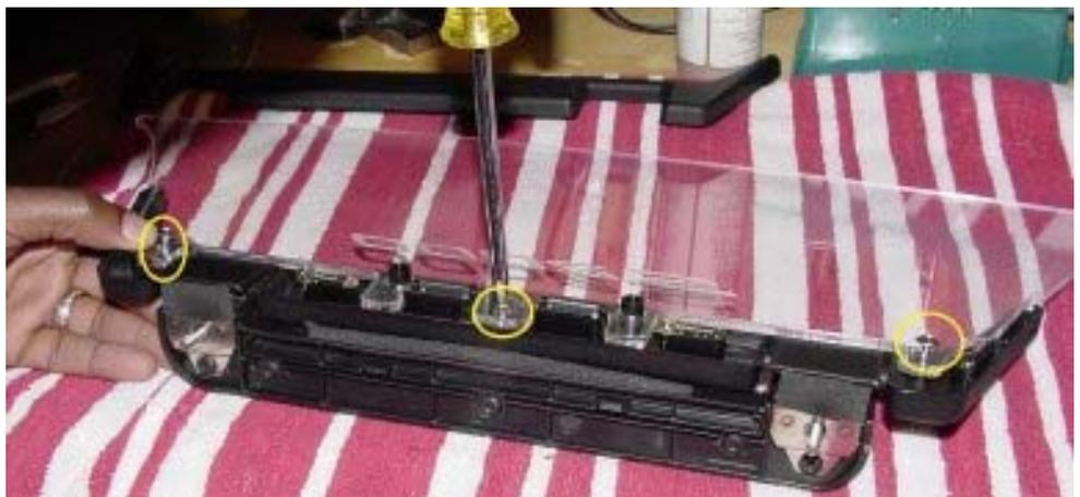
10. Now take the Goop (available at Home Depot or any hardware or housewares store) and place a generous dab on each of the slots into which the tabs on the opposite side of the mechanism fit. Also place a thin thread of of superglue around the perimeter of each ear all the way down to the base and around the bottom corners to the hinge. Be careful not to
